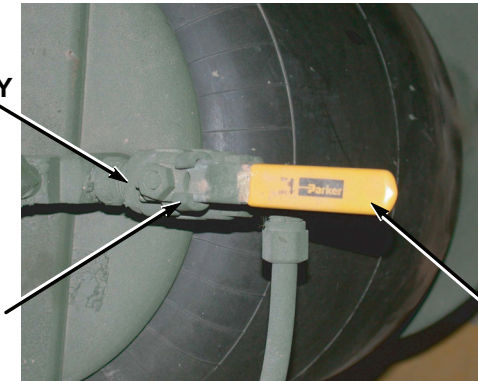
BALL VALVE SHOWN IN ON POSITION
